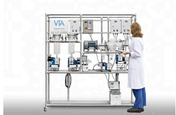
Figure 3: Horizontal Laboratory Evaporator
